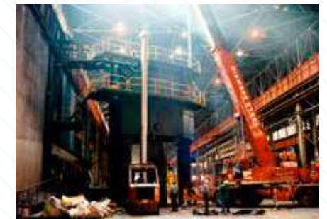
The world's largest bolt-style Superbolt being installed in a two-post hydraulic forging press.
