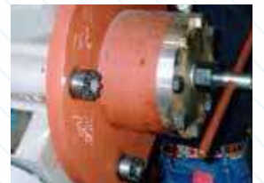
MT Tensioner on Cylinder Heads
